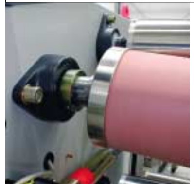
Bearing arrangement of bow roller
