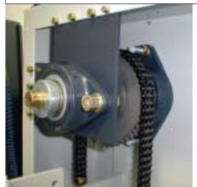
Double-chain drive of bow roller
