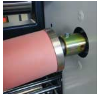
Bearing arrangement of bow roller (drive end)
